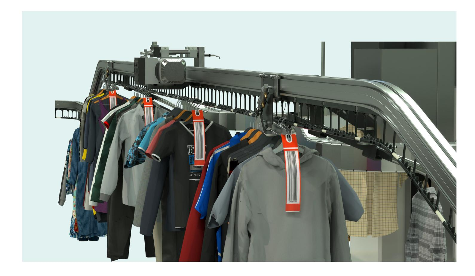
Identifies the transported goods through labels, separation hangers, or barcodes. It is ideal for continuous use in hanging garment installations, thanks to its three-dimensional movement of garments and minimal maintenance requirements.
