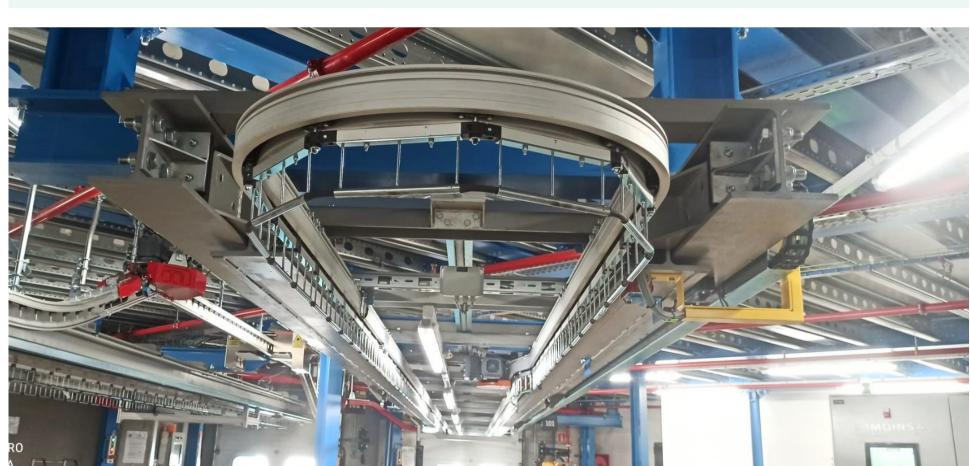
Enables the connection between flows with different cadences by facilitating the accumulation of garments before moving to the next stage of the process.
